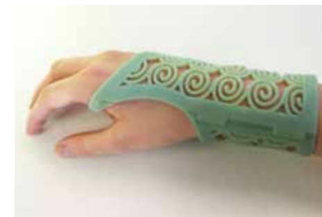
Figure 2. 'Swirl' splint built using ABS-like material on an Objet Connex PolyJet machine
